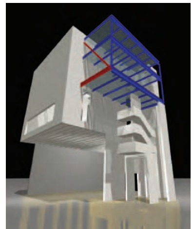
Computer rendering showing concrete and steel structure of the Unicorn Theatre, London, concealed by cladding in the finished building.
